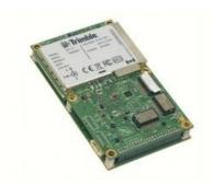
Applanix, a Trimble company, has introduced the Trimble AP+ Air OEM solution for direct georeferencing of airborne sensor data. The solution enables users to accurately and efficiently produce maps and 3D models without the use of ground control points.
