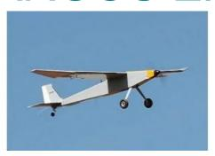
CATUAV, Spain, has developed an electric version of the ARGOS UAV platform designed specifically to meet the demands of CSIC's MESTRAL project. This new platform will enable images to be obtained simultaneously in the thermal, NIR and visible spectrums in Alfacs Bay in a single one-hour flight.
