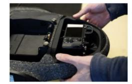
Atmos has integrated Sony  $\alpha$ 7R mark III and IV cameras into its drones to increase the coverage and accuracy achieved in a single flight. The Dutch manufacturer of high-end vertical takeoff and landing (VTOL) fixed-wing drones (Marlyn Cobalt) for surveying and mapping applications regards this as a new milestone in its drone development work.
