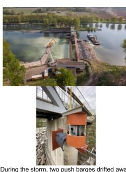
Automated movement detection supports informed decisions about infrastructure, including for waterways as illustrated by this project in the Netherlands. Following storm-related damage to a weir on the River Maas, Trimble dealer Geometius quickly helped to set up a real-time automated system. It monitored the weir 24/7 to give stakeholders advance warning of potential catastrophe in the case of excessive movement.
