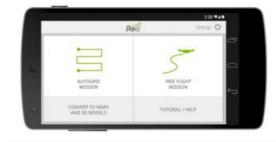
Making use of DJI's new DJI Phantom software development kit, Pix4D has developed the first mapping app: the Pix4Dmapper mobile app allows drones such as DJI Phantom 2 Vision to be turned into an autonomous mapping and measuring tool for creation of 2D maps and 3D models.
