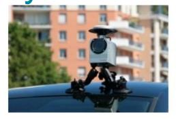
The Belgian Road Research Centre (BRRC) has recently chosen imajbox, a mobile mapping system from imajing, to perform road network condition assessment and monitoring and keep memory of field status. imajbox can be installed on various vehicles in order to record field data which will be valuable for results interpretation and validation.
