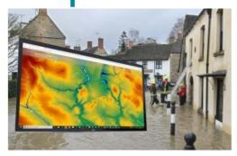
3D models derived from high-resolution aerial photography are underpinning the most upto-date flood risk map of the UK. Working alongside Ambiental Risk Analytics (ARA), aerial mapping company Bluesky has supplied photogrammetrically derived digital terrain models (DTMs) for the whole of England, Scotland and Wales. Combined with river flow and rainfall data, these 3D models allow ARA to deliver a range of flood risk information for any property in the UK.
