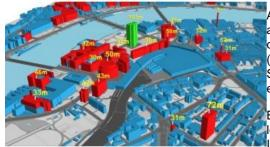
Aerial mapping company Bluesky has launched the first UK nationwide map providing accurate height measurements for around 40 million buildings. Created from a combination of remote sensing surveys, including data from aircraft mounted lasers (Lidar), the Bluesky Heighted Building dataset covers the whole of England, Wales and Scotland, and will help to change the way we visualise and understand the built environment.
