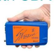
The SXBlue II GNSS from Geneq, Canada, is a GNSS receiver that uses both GPS and GLONASS with SBAS (WAAS/ EGNOS/ MSAS/ GAGAN) to attain 30cm/1ft (RMS) accuracy in real-time using free SBAS corrections. It connects through Bluetooth to any smartphone, handheld, tablet computer or notebook computer.
