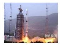
A Chinese CZ-4C Chang Zheng-4C launch vehicle - carrying the Feng Yun-3A satellite - has lifted off from the Taiyuan Satellite Launch Center located in the Shanxi province. The first satellite of the second generation of polar orbiting meteorological satellites will operate in a 836 km sun-synchronous orbit with an inclination of 98.7 degrees, covering the planet twice a day.
