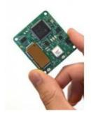
Cambridge Consultants, a British developer of innovative products, has announced a new technology that can accurately detect someone's location indoors when GPS drops out. A number of sensors and a custom algorithm determine the location, with an accuracy of within approximately 1% of the distance travelled. The technology uses low-power, low-cost sensors and the device concept is small enough to clip onto a belt. Furthermore, it requires no existing internal infrastructure.
