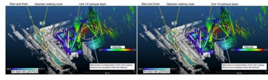
The Japan Atomic Energy Agency (JAEA) successfully developed a way to 3D scan and visualize the radiation data from the 2011 Fukushima nuclear disaster by combining a Compton camera, radiation meter and Kaarta Stencil 2 mobile mapping system.
