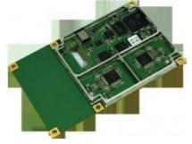
Hemisphere GNSS has launched its new Crescent Vector H200 GNSS compass module, a high-performance receiver for heading, positioning, heave and attitude. Vector H200 is designed for professional marine, navigation and land applications in challenging and dynamic environments.
