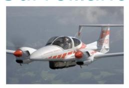
Diamond Airborne Sensing recently received certification for the DA42 MPP in surveillance and laser scanning configuration for Russia. The DA42 MPP is able to carry daylight and thermal cameras, and is linked to ground stations with satcom and/or line of sight downlink systems. Survey equipment, such as LIDAR or hyperspectral scanners and digital cameras, can be carried in the belly pod underneath the fuselage.
