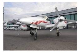
Displaying 21 aerodynamical improvements, the newly developed DA42 V1 marks another milestone in the history of Diamond Aircraft Austria. The top speed of the aircraft is over 200 knots in FL180 (18,000ft), and the DA42 is often used for remote-sensing survey flights.
