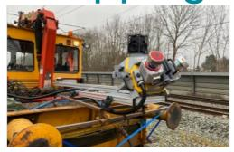
Trimble's MX9 mobile mapping system is the first ever vehicle-independent mobile mapping system officially approved by German national railway company Deutsche Bahn for surveying tracks, points, clearances and topographic objects.
