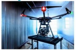
DJI has introduced the Matrice 600, its next-generation aerial platform, developed for professional aerial photography, filmmaking and industrial applications. The M600 integrates DJI's brand-new A3 flight controller onboard and features advanced Lightbridge 2 video-transmission technology that offers high frame rates and HD live-streaming capability at distances up to five kilometres.
