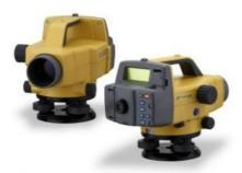
The Topcon DL-500 implements †Wave-and-Read' technology, providing an additional survey style option that allows a rod person to wave the staff back and forth, instead of keeping the staff plumb. The staff reading becomes the minimum when it stands vertically. The DL-500 tracks the waved staff and automatically reads the least value. This allows for error-free readings, while eliminating eyestrain.
