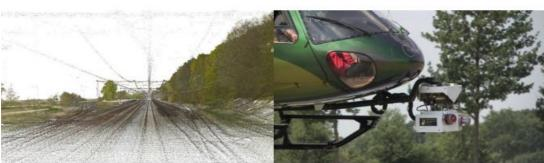
ProRail, the company in charge of managing and maintaining the Netherlands' railways, is using 3D aerial imagery to reduce travel disruption. The company has scanned more than 7,000km of railway tracks over recent months, and the imaging project is due to be completed this summer. The resulting Lidar images will
