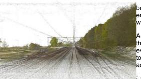
be used to produce a detailed 3D map which will help to minimise delays by enabling ProRail employees to see areas of track that need replacing or where trees need to be cut down.
