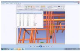
ClearEdge3D has released EdgeWise Plant 3.0 including six major new features to optimise and accelerate 3D modelling workflows. The software automates the extraction of complex CAD pipe geometry from 3D laser scanned data, dramatically reducing the time needed to create accurate asbuilt 3D models of process plant facilities.
