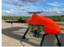
Topodrone has announced the integration of its Lidar Prime scanner with the aOrion Heli-E UAV enabled by Velodyne's Alpha Prime sensor. This is aimed at bridging the gap in UAV-based mapping solutions between heavyweight and expensive manned aerial Lidar systems and lightweight drone Lidar systems. The system allows users to expand their applications to survey large areas that
