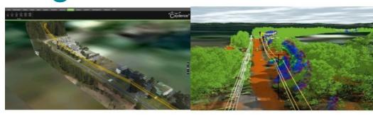
Australian energy distributor Essential Energy has contracted NM Group to map, analyse and report on vegetation risks which could pose future safety and reliability issues across its overhead electricity network. The programme will use innovative remote sensing and 3D modelling technologies around nearly 85,000km of powerline. This will enable improved prioritisation and planning of
