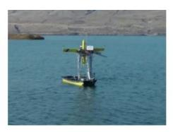
The newest aircraft carrier does not have acres of flight deck. In fact, it has no deck at all. Rather than carrying a crew of thousands, it sails without a soul on board. Yet the aircraft that it operates can fly much longer and further than anything based on a fleet leviathan. That aircraft is Aerovel's 20kg Flexrotor, which combines VTOL and a small footprint with a Hawaii-to-West Coast range. The carrier is a 4-metre skiff equipped to launch, retrieve and service the Flexrotor automatically.
