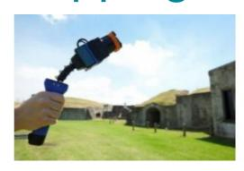
Australian researchers are using the novel mobile laser 3D mapping system called Zebedee to preserve some of the country's oldest and most culturally significant heritage sites. The handheld 3D mapping system is developed by CSIRO and can scan an environment as an operator walks through it.
