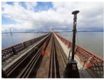
Fugro has been awarded a contract to survey Scotland's entire rail network and provide Network Rail with a holistic gauging database that includes clearance data from the track to lineside structures, platforms, objects and the train-to-train passing interface. The routewide gauging geodata will support the continued safe passage of trains operating on the network and facilitate the introduction of new rolling stock.
