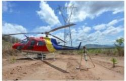
South Africa-based GeoM has completed an aerial survey project of overhead power lines in Angola. Using a helicopter-mounted high-speed laser scanner, complete with advanced navigation and positioning system, GeoM captured around 1,500 kilometres of detailed Lidar measurements. Complemented with high-resolution aerial photography and meteorological data, the laser-scanned point cloud will be used by the power company's engineering department to support maintenance and upgrade programmes.
