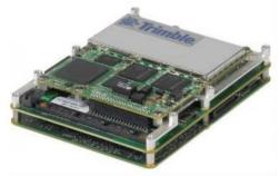
Trimble (USA) has added the AP20-C to its AP Series of embedded GNSS-Inertial OEM boards plus Inertial Measurement Unit (IMU). Using a compact, custom-built IMU based on commercial Micro Electromechanical Machined (MEMS) inertial sensors, the AP20-C enables system integrators to achieve high-rate position and orientation measurements with exceptional accuracy.
