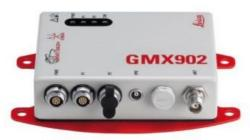
Leica Geosystems' GMX902 family of streamlined receivers for deformation monitoring and real-time reference station applications has been extended with the GMX902 GNSS. This device offers 50Hz data rate, triple frequency and Galileo tracking. Additionally the existing GMX902 GG has been updated with high-speed serial ports and even lower power consumption than before.
