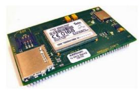
Aldacom presents the AldaLogic C10/3, a breadboard which contains a complete embedded Linux PC on a surface of just 104mm x 63mm. A Quadband GPRS module and SiRF3 GPS module are also on board, as well as interfaces for USB, RS232 and Ethernet components. An SD-card reader enables the trouble-free expansion of the 4 Mb of flash memory which comes as standard.
