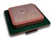
Tallysman Wireless has released the TW5115 Embedded Smart Antenna/Receiver. It features the STMicroelectronics STA8058 Teseo WAAS, EGNOS and MSAS-enabled GPS L1 receiver IC, a high-performance, low-noise amplifier stage, a tight out-of-band BAR pre-filter to reject interference, and a perfectly tuned antenna element for maximum GPS signal reception, even in dense urban-canyon environments where multipath interference is prevalent, according to the manufacturer.
