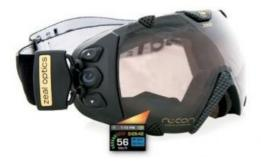
The Zeal Optics Transcend GPS Goggle enables skiers to monitor their speed and altitude, as well as the time and vertical speed, using the GPS Goggle. The various data are visible on a head-up display. The stats can be downloaded on your computer with a Google Map overlay to review performance. The rechangeable lithion-ion battery allows 7 hours run time.
