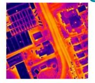
An aircraft fitted with specially developed survey equipment is taking to the skies over Britain\'s cities at night. Using a new super-sensitive thermal sensor, Leicestershire-based aerial mapping company Bluesky is capturing highly accurate measurements of heat loss from buildings. The results of these night-time thermal surveys will provide local authorities, energy providers and even householders with intelligence to tackle energy inefficiency and fuel poverty.
