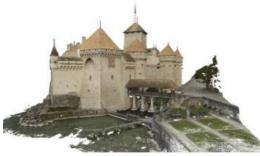
Pix4D has created a highly accurate and very dense 3D model of Chillon Castle (Château de Chillon), Switzerland's most visited historic monument. The 3D point cloud integrates the indoor and outdoor structures of this highly complex architectural object with a resolution of up to 5mm. It is based on both aerial and terrestrial images captured using DJI Phantom 2 Vision, GoPro Hero 3+, Canon 6D and Sony alpha 7r cameras with fisheye lenses.
