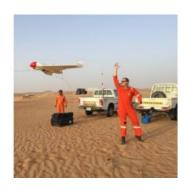
Skeye from The Netherlands and Fugro Maps recently completed an aerial topographic survey using a fixed-wing UAV in the desert south of Abu Dhabi in the United Arab Emirates. Fugro's client insisted on rapid project execution meaning that the survey was carried out in the middle of summer. With measured temperatures in the sun of up to 68 degrees Celsius this must be one of the hottest UAV surveys ever conducted.
