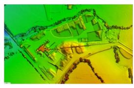
Unmanned aerial vehicles (UAVs or 'drones') are a powerful tool for stockpile measurement in industries such as mining, forestry and construction. They allow the same region to be flown regularly and progression of the work to be monitored over time. Imagery is collected over the region of interest at high resolution,
