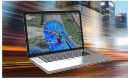
IDS GeoRadar, part of Hexagon, has enhanced IQMaps, its post-processing software application for advanced GPR data analysis. The updated version includes new functionalities that improve the visualization of radar data and extend the application fields to void detection and archaeology.
