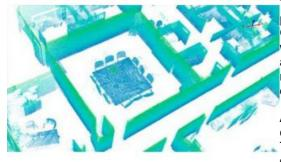
Trimble's Indoor Mobile Mapping System (TIMMS) is a manually operated push-cart designed to accurately model interior spaces without accessing GPS. It consists of 3 core elements: Lidar and camera systems engineered to work indoors in mobile mode, computers and electronics for completing data acquisition, and data processing workflow for producing final 2D/3D maps and models. The models are geolocated, meaning that the real-world position of each area is known.
