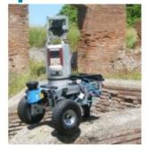
Motivated by the increasing need for rapid characterisation of environments in 3D, a German university has designed a robot system that automates the work of an operator of terrestrial laser scanners. The system makes it possible to work without markers or targets, saving surveyors more than 75% of the time spent on site. Another impulse for developing the platform was the demand for a remote inspection tool.
