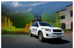
The IP-S2 HD Mapping System is a vehicle-mounted surveying and mapping system featuring a high-definition Lidar scanner from Velodyne Lidar. The IP-S2 HD Mapping System incorporates Velodyne's HDL-64E S2.2 Lidar scanner, allowing vehicle operators to acquire very dense point clouds while travelling at posted speed limits even in inclement weather.
