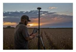
Juniper Systems has introduced the all-new Geode GNS3 GNSS receiver. It enables users to easily collect real-time GNSS data with sub-metre, sub-foot and decimetre accuracy options – without the huge price tag or complexity of other precision receivers. This scalable platform allows users to purchase the level of accuracy they need now while having the option to increase accuracy in the future. The Geode GNS3 GNSS receiver is now available worldwide.
