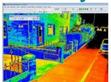
The new Leica Cyclone v7.1, a significant advance in Leica Geosystems Cyclone point cloud software, speeds these key office steps: (1) accurately registering multiple scans together and (2) navigating to and clearly visualizing specific areas of interest.
