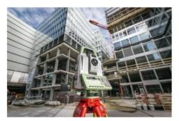
Leica Geosystems, part of Hexagon, has unveiled the new Leica Nova MS60. According to the company, the MS60 MultiStation brings sensor fusion to the next level by combining upgraded faster 3D laser scanning capabilities, GNSS connectivity and digital imaging with a highest-end total station.
