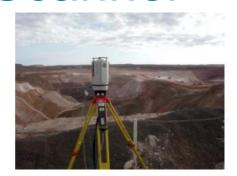
The RIEGL VZ-1000 high-performance Terrestrial Laser Scanner for long range applications is launched at INTERGEO 2010 in Cologne. The scanner is especially qualified for surveying in open pit mining. The RIEGL VZ-1000 offers a very long range up to 1400m, in combination with high-accuracy and high-precision, while still operating in Laser Class 1.
