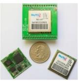
SkyTraq Technology, a Taiwanese GNSS positioning technology company, has introduced S2525F8-RTK, a low-cost, low-power, single-frequency RTK receiver for applications requiring centimetre-level accuracy positioning. The multi-constellation GNSS RTK receiver can use 12 GPS, eight SBAS and six BDS signals and one QZSS signal. In situations where RTK fix is not possible, a Float RTK mode can be used for decimetrelevel accuracy positioning.
