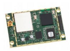
NovAtel is pleased to announce that the 1.011 Firmware Release for its OEMStar L1 GNSS receiver has significantly reduced the card's power consumption. The receiver now consumes only 450mW for GPS+GLONASS operation and 360mW for GPS-only operation.
