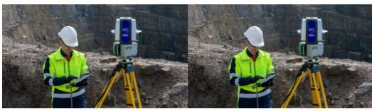
A new dual-window scanner that halves data capture time headlines the latest Maptek mine measurement improvements. The new Maptek XR3-D mkll laser scanner with dual-window arrangement is designed to cut scan acquisition time in half. Whereas conventional terrestrial laser scanners capture data from one window, spinning to achieve a 360° field of view, the XR3-D
