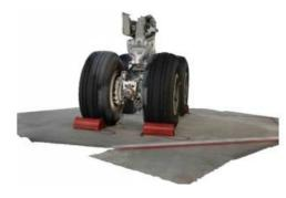
Surveyors Uli Bauer and Andreas Gelhausen have generated a 3D model of the landing gear of the zero-gravity Airbus A300 ZERO-G – used to perform parabola flights for scientific purposes – that is accurate to +/-5mm. Furthermore, they have used the Aibot X6 UAV to generate a point cloud of the aircraft.
