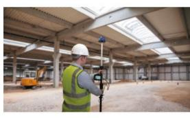
Racelogic has launched a brand-new indoor positioning system, called VIPS, which is an advanced system for measuring real-time 3D position to an accuracy of ±2cm in areas where GPS is not available. This makes it an ideal tool for construction applications both indoors and in urban areas. The system has been designed for any application that requires accurate measurement and recording of 3D positioning. It enables GPS-based technologies to operate in GPS-denied environments.
