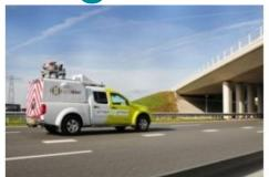
Geomaat, a Dutch company specialised in geodetic survey services, has developed a method of measuring safety barrier heights on European roads. The system uses StreetMapper, 3D Laser Mapping's mobile laser mapping system, and automated feature extraction software. This combination makes it possible to process laser scanned point clouds to determine the height of existing barriers.
