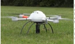
Microdrones has announced the release of a professional aerial methane detection solution, the <a href="mailto:mdTector1000 CH4">mdTector1000 CH4</a>. The solution has a Pergam gas sensor, mounted and integrated with the UAV. In real time, you will be able to see aerial shots of what you are detecting with the laser sensor and you can easily navigate terrain that's too dangerous for traditional foot crews.
